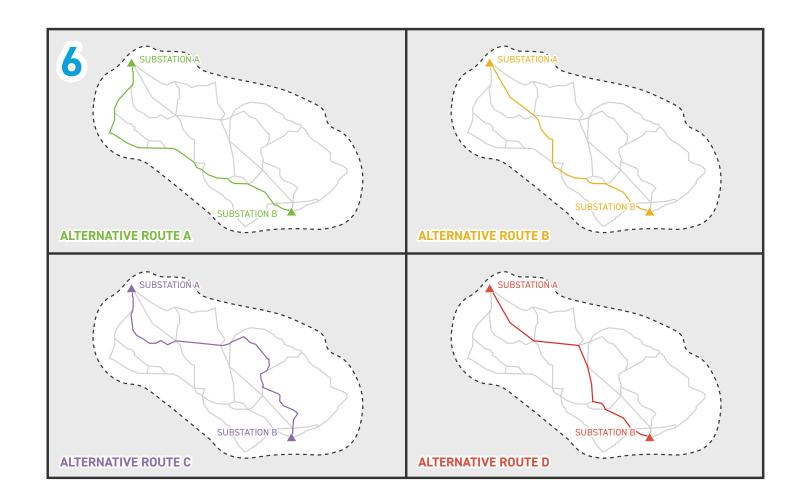
6. Alternative Routes: After public input is gathered, study segments are further refined and evaluated. The most suitable segments are selected and assembled into alternative route options.
